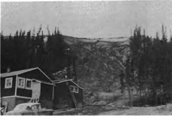
Figure 6. Mud flows on escarpment, east end of cross runway, May 1957. (Note snow drift at top of scalloped portion (DBR photo BR 6762))
